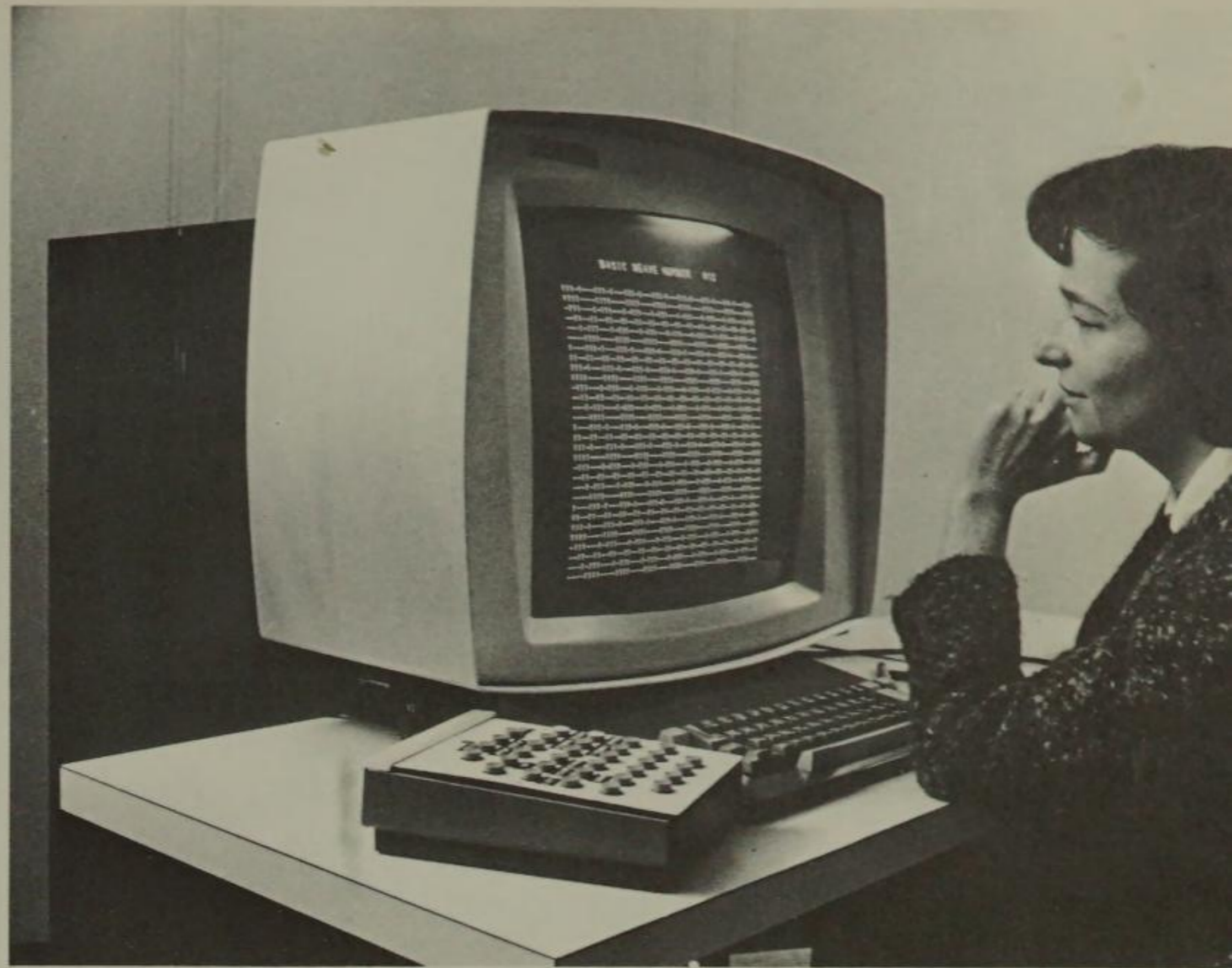
5-34. Dr. Lourie in front of the cathode ray tube before she begins her design. She selects a weave design from a library of hundreds of weaves previously stored in the computer. (Photographs 5-34—5-35F reproduced courtesy IBM Data Processing Division.)
