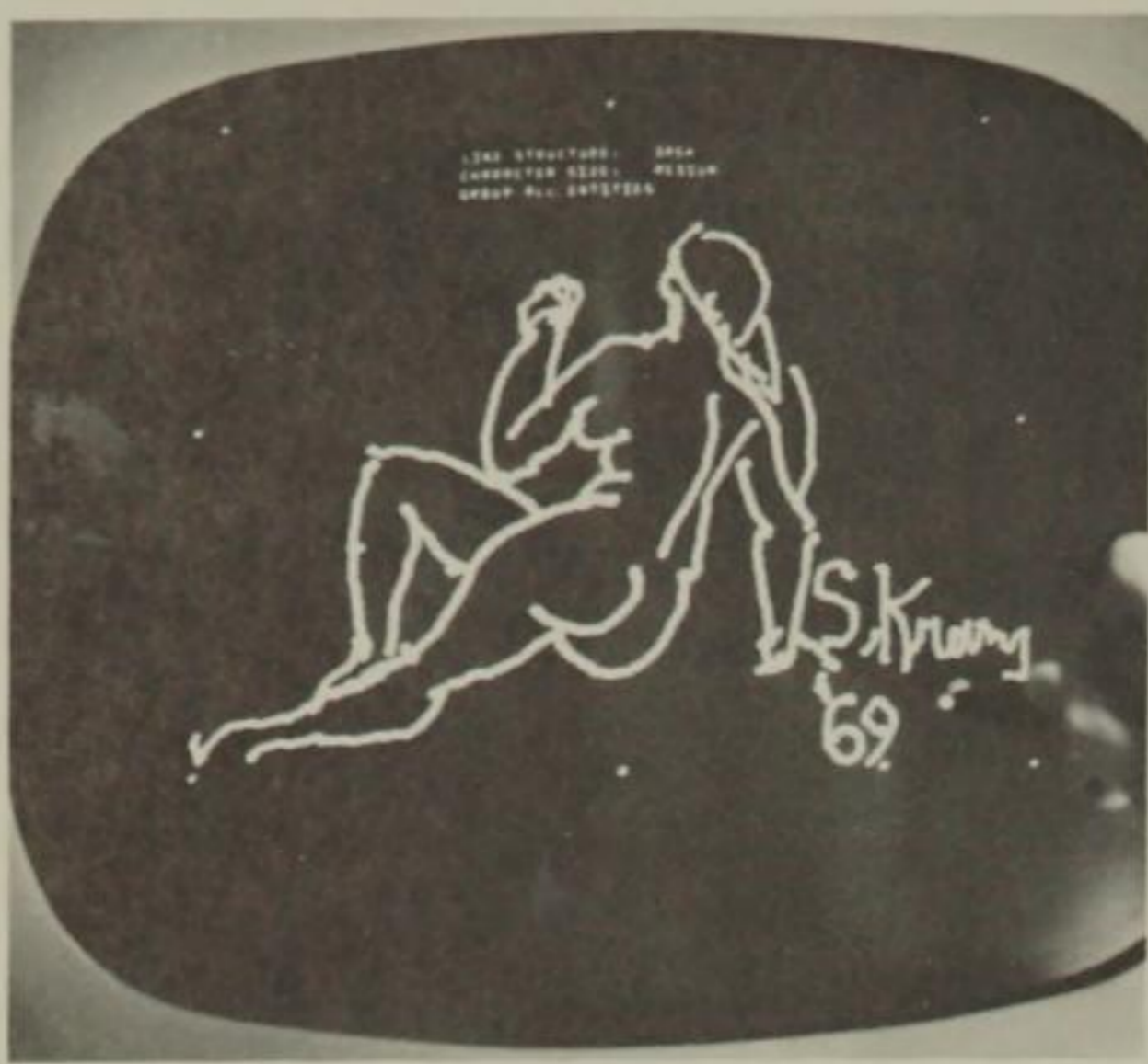
5-24A. The author used a light pen to make this free-form line drawing directly on the face of the cathode-ray tube. The light pen makes a series of very short, straight lines on the tube, and that input is taken into the computer memory bank, where it is retained.
