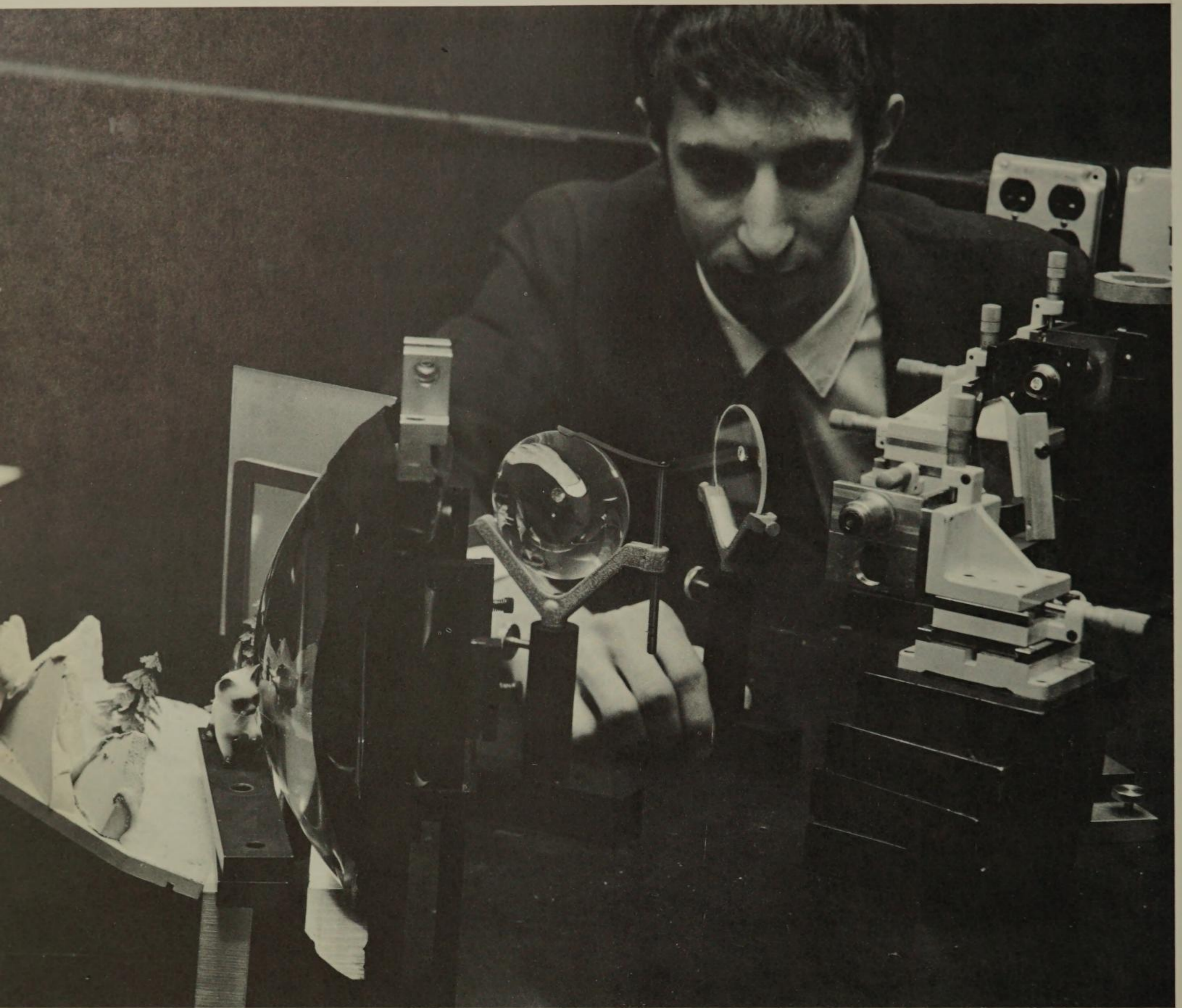
4-23. Gabor's assistant in the laboratory. The photograph shows the setup used for Gabor's experiment in three-dimensional holography. Note the set at the lower left of the photograph. (Courtesy CBS Laboratories, Stamford, Connecticut.)
