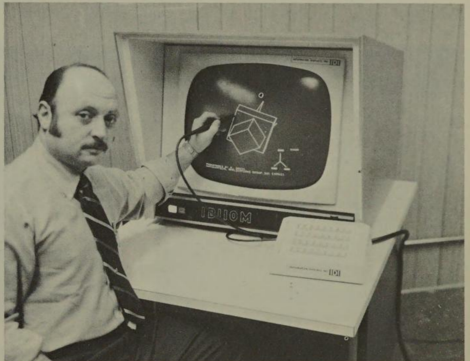
5-22. Carl Machover working with a light pen on the face of a cathode-ray tube, to be used as a graphic input for a computer program.
