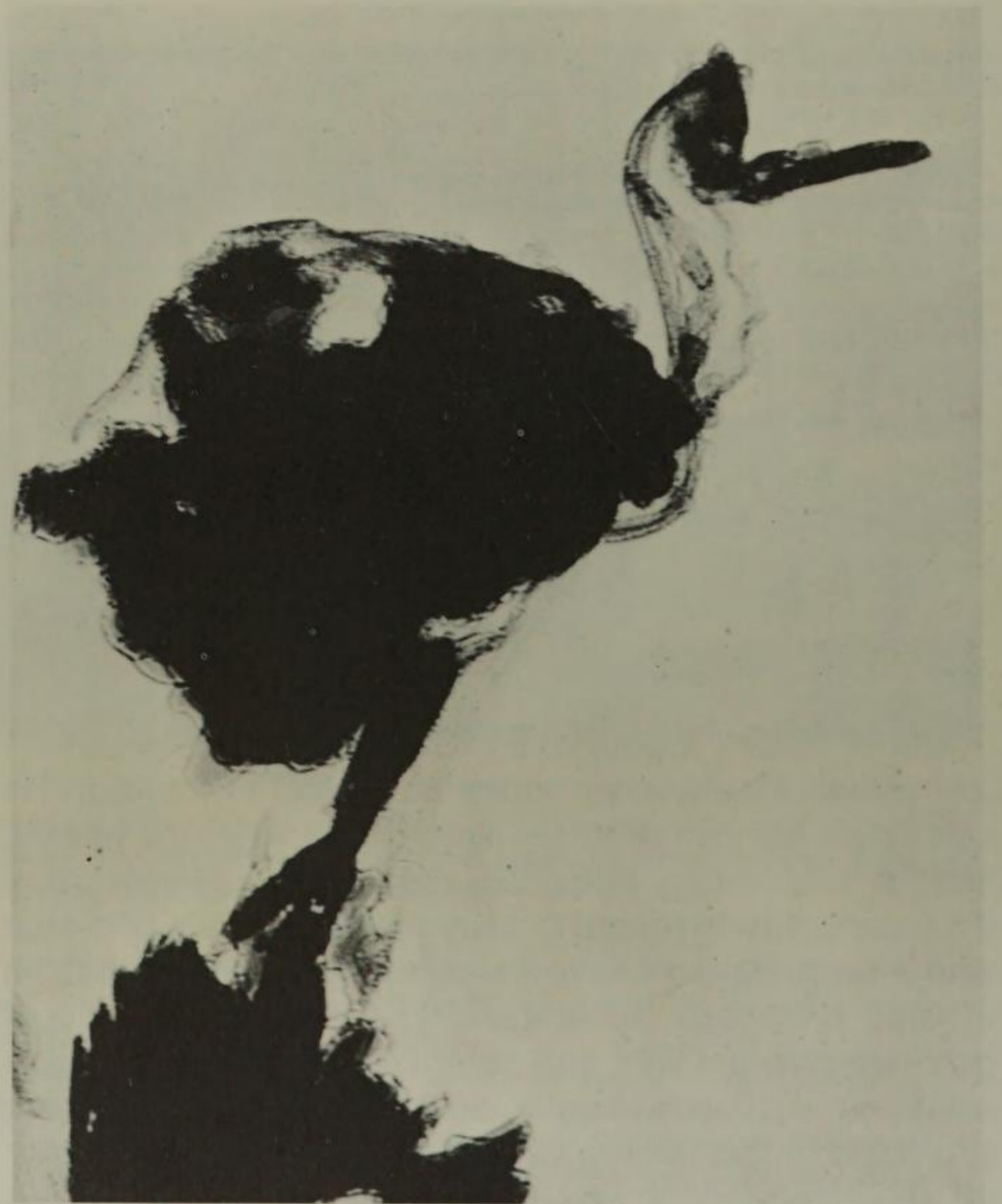
4-11. Kaolin particles on torn formvar supporting membrane. By chance, under the impact of the electron beam, the particles assumed the shape of a bird. Magnification: 10,000X. Taken with a Czechoslovakian electron microscope, TESLA. (Courtesy Dr. Bystricky.)
