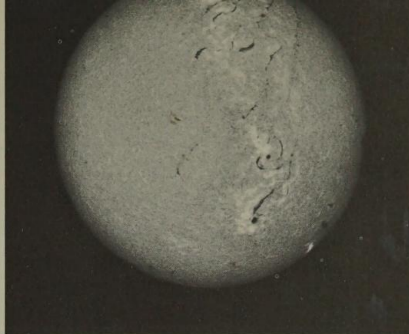
4-38. A photograph of the sun taken in the light of the red hydrogen line with a Zeiss (Oberkochen, West Germany) H-alpha Monochromator. (Courtesy Carl Zeiss, Inc., New York.)
