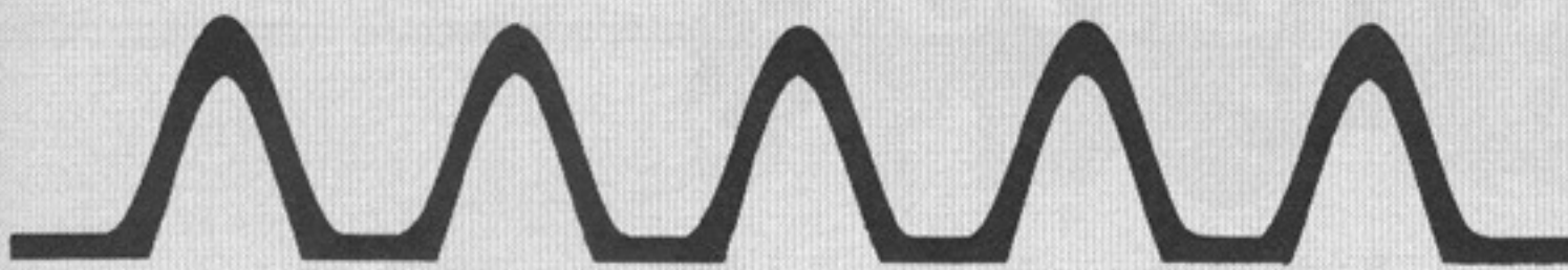
Figure 2. Output of vocal oscillator.
