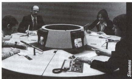
The problems of video-phone conferencing are being studied in trial tests. The photo shows one of the conference tables designed for this purpose, with additional equipment for the conference director in the foreground.
